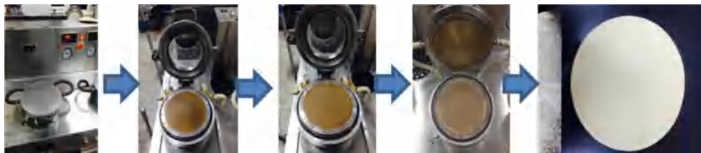
Fig. 8. The brief schematic diagram of the process of the paper-making.
