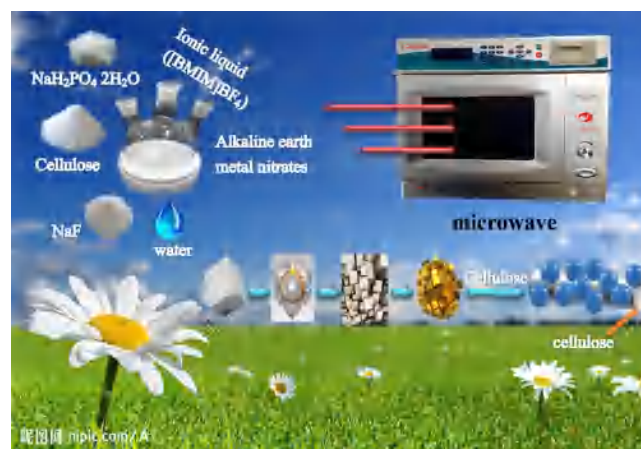
Fig. 1. The schematic diagram of the formation process of cellulose/alkaline earth metal fluorides particles.
